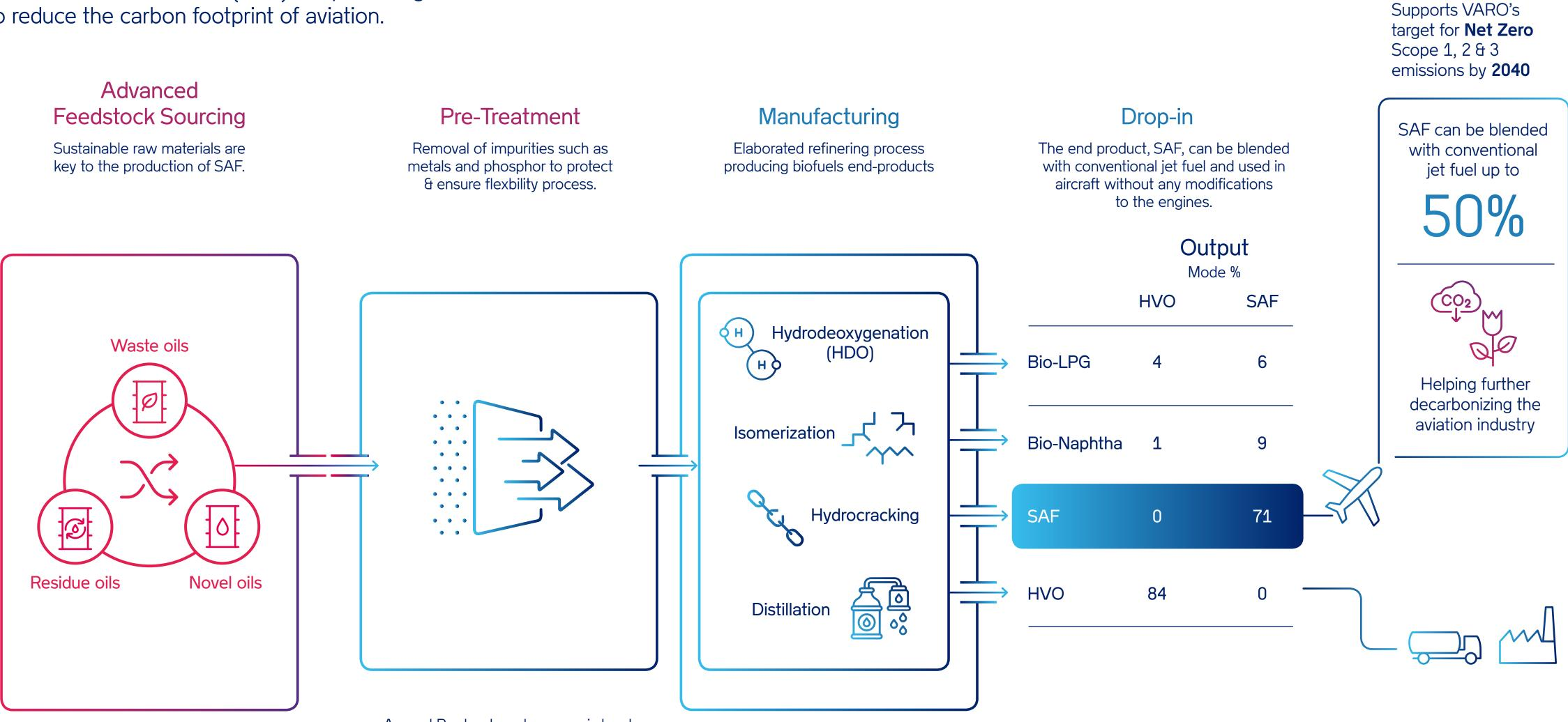
A good Pre-treatment process is key to the flexibility of the feedstock sourcing.
